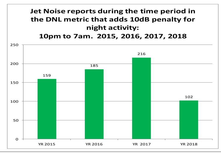
This data underscores the intrusion of noise during what might be called quiet times. In conducting a Day/Night Average Sound Level (DNL), a 10 dB correction is applied to nighttime (10:00 p.m. and 7:00 a.m.) sound levels to account for increased annoyance due to noise during the night hours.
